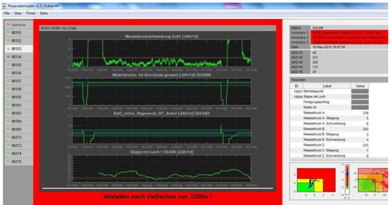
Figure 2. An HMI based on MATLAB that enables equipment operators to receive warnings about potential failures before they occur. © 1984–2019 The MathWorks, Inc.
